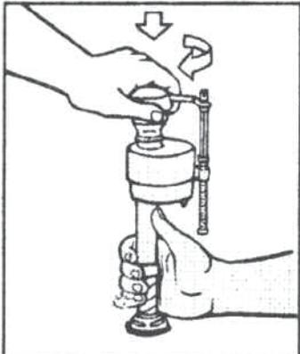
**DIAGRAM 3:** Replace TOP by engaging lugs and rotating 1/8 turn clockwise. **MAKE CERTAIN TIP IS TURNED TO THE LOCKED POSITION.** VALVE MAY NOT TURN ON IF TOP IS NOT FULLY TURNED TO THE LOCKED POSITION.
