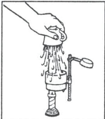
**DIAGRAM 2:** While holding a container over the uncapped VALVE to prevent splashing, turn water supply on and off a few times. Leave water supply off.
